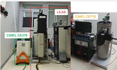
Fig. 1. CIMEL CE376 micro-pulse lidar, LILAS high-power lidar and CE710 high-power CIMEL lidar at ATOLL platform
